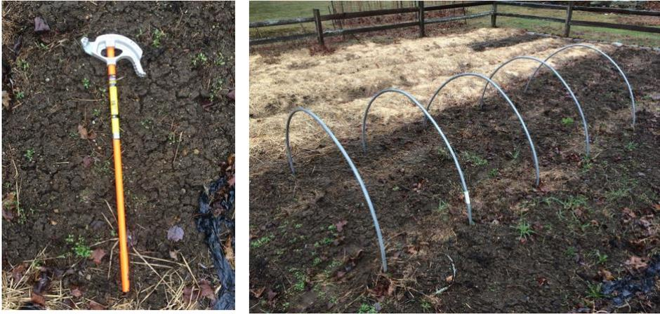
Fig. 6. An electrical conduit bender, which can be used to create metal hoops from ten foot lengths of conduit. Metal hoops are very strong, but they do need to be secured enough to prevent them from falling over. They may also be more costly than PVC hoops because of the need to purchase a bending tool.
